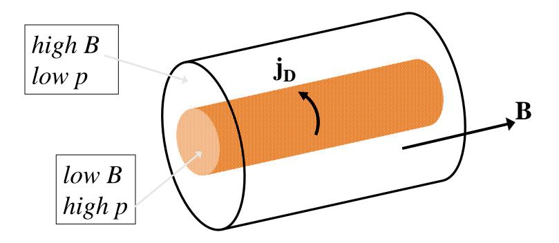
• The diamagnetic current  $j_D$  decreases the magnetic field inside the plasma keeping the sum of thermal and magnetic pressures constant everywhere in the cylinder
